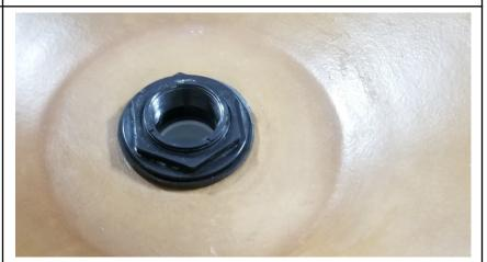
4. First place the foam gasket over the flange. Second place the washer on top of the foam gasket. Third thread the nut to the flange
