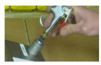
Step 4. Reduce the compressor output pressure (10 to 20 psi). Place one hand on the Outlet side of the valve while injecting air into the Inlet side of the valve. If you have cleared the debris – you will not feel any air coming out of the Outlet side of the valve. If you do feel air, repeat the steps above. If after repeated attempts you still cannot clear the debris, the AWEIS valve box must be replaced. **Normally the debris will clear after the first attempt.**
