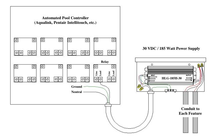
Wiring to Pool Controller when 2 Features Turned ON separately
