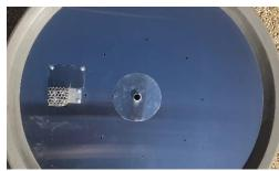
9. Install the burner onto the pipe nipple coming up through the center of the pan as shown in the photo at right.
