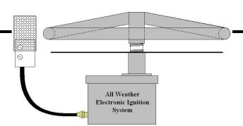
All Weather Electronic Ignition Field Serviceable (30 VDC) Commercial Grade System
